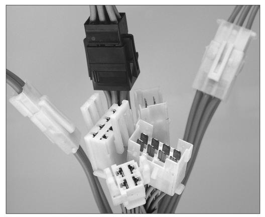
In an effort to overcome the problems arising from the careless mating of connectors during assembly, the Positive Mate connector is designed so that a condition of partial engagement is impossible.
