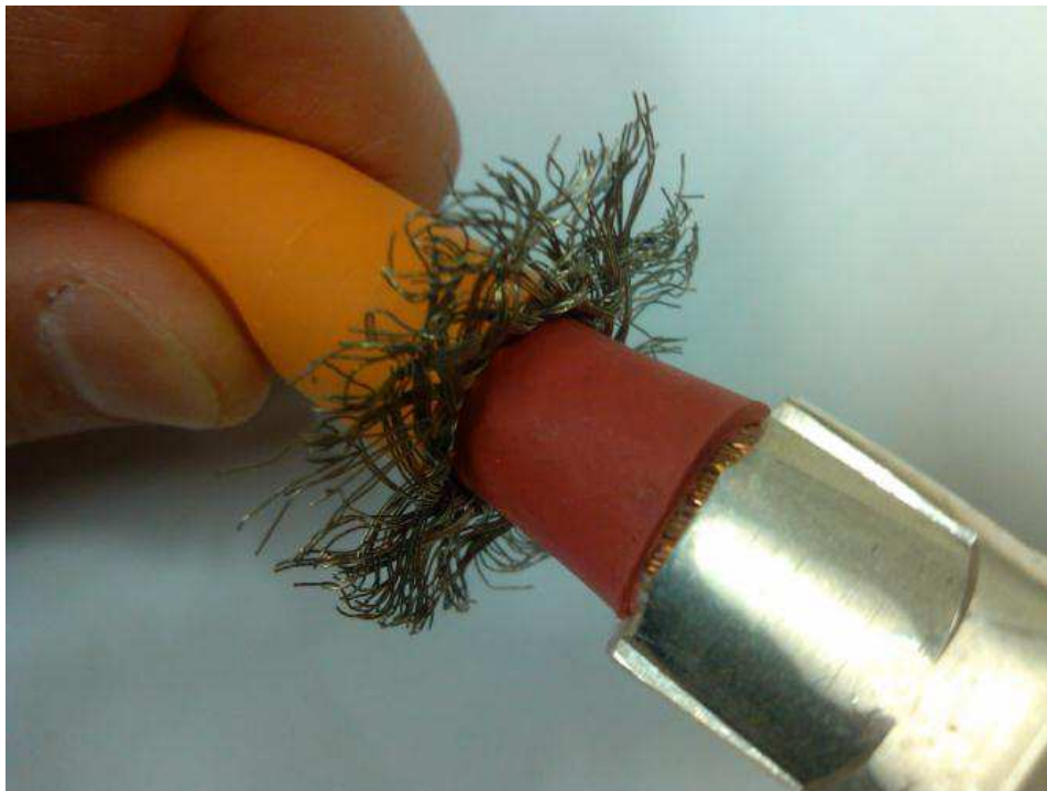
Figure 5: Hackle the shield braid
