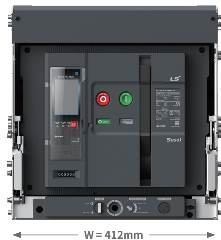
E-Frame ~ 4000AF 75kA @900VAC* 50kA @1150V
