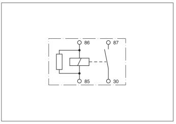
Polarity: Terminal 86 and terminal 30 to +
