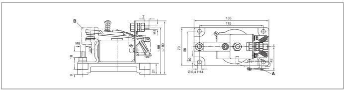
Accessories: Tyco (AMP) Supersal connector; Connector housing no. 282080-1; Contact no. 183025-1 (x2); Single wire seal no. 828920-1 for 1.5mm² cable (x2)
