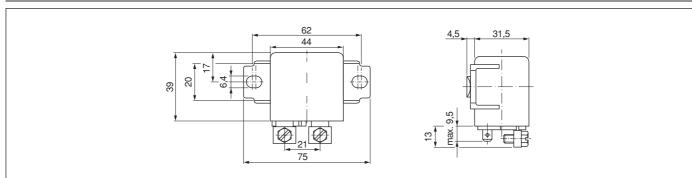
Accessories: Double receptacle housing for excitation side (terminals 85 and 86). Order using Tyco (AMP) number 180 907 from: Tyco (AMP) Deutschland GmbH, Amperestraße 7-11, D-63225 Langen, Tel. 0 61 03/70 90.
